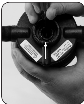
Step 4. Remove #17 O-ring and replace.
