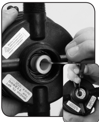
Step 7. Replace #82 SHAFT SEAL SPACER and #16 Gasket.
