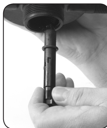
Step 6. Re-install #52 UPPER SHAFT and #17 O-ring.
