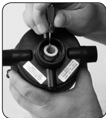
Step 4. Remove #82 SHAFT SEAL SPACER.
