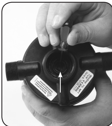
Step 5. Remove #17 O-ring and replace.
