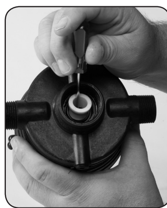
Step 3. Remove #83 SHAFT SEAL SPACER.
