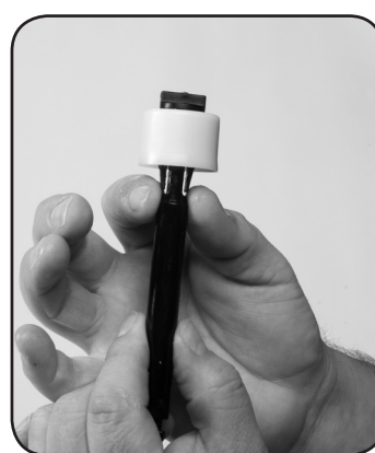
Step 6. Squeeze ears on shaft and remove #44 DOSAGE PISTON.
