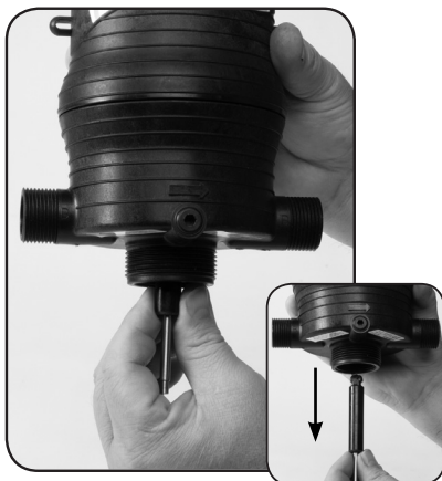
Step 2. 1/4 turn to remove #51 SHAFT ASSEMBLY
