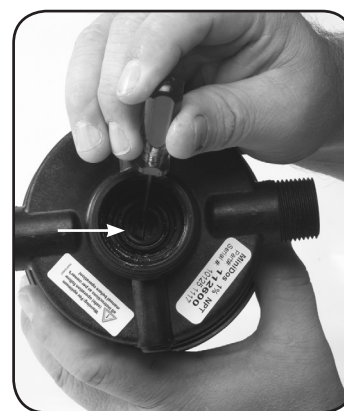
Step 6. Replace #17 O-ring.
