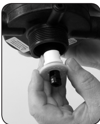
Step 7. Re-install #82 SEAL SPACER and #16 GASKET.
