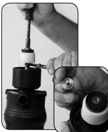
Step 2. Unscrew to unlock and remove #93 CAPSCREW.
