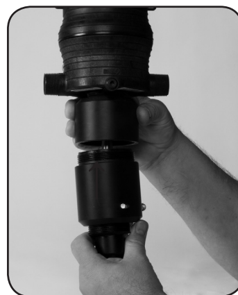
Step 9. Screw #61 OUTER CYLINDER onto body.
