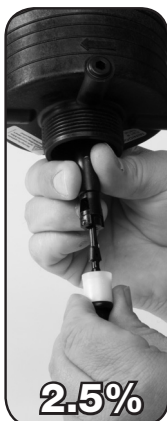
Step 2. Rotate #51 or #52 SHAFT 90° and remove.
