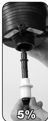
Step 2. Rotate #51 or #52 SHAFT 90° and remove.
