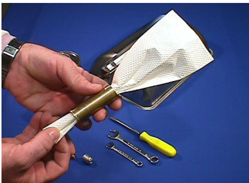
17. With a soft cloth or paper towel, clean the interior wall of the brass venturi.
