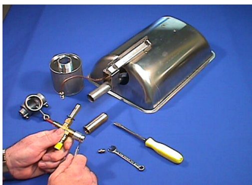
12. Attach your 13 mm wrench to the hex head on the interior coil cover. Warning! The gas supply must be cut off prior to performing this step.
