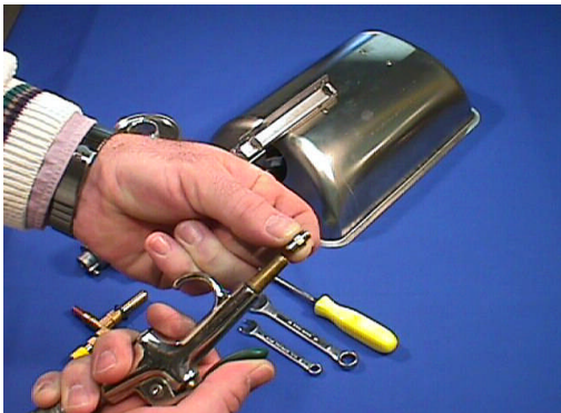
15. To clean the jet orifice apply compressed air to both ends of the jet. Warning! Never insert any object into the orifice to dislodge foreign material.
