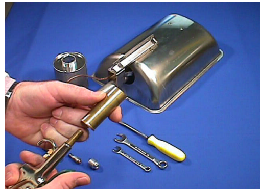
16. To clean the brass venturi, first blow out the interior with compressed air.
