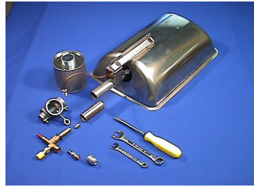
14. You have now disassembled the heater enough to perform a general cleaning and inspection.
