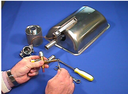
10. Grasp the safety device/jet holder assembly, taking care to not put pressure against the by-pass button. Attach your 5/16" or 8mm wrench to the hex head on the jet.
