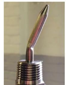
*A bend in the probe will limit movement of the internal parts*
