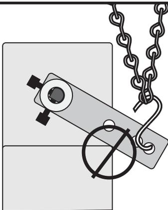
Do not allow the motor arm to be stopped or hindered by the motor body.
