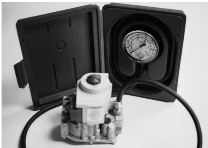
Valve shown is outside of heater for clarity of view.
