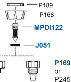
**!** Using tools could damage the plunger and affect the injection rate
