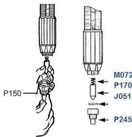
6. Insert new white stem into black sleeve, making sure black key in sleeve is aligned with long groove in stem.
