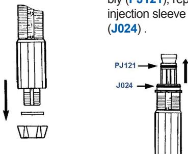
8. Replace check valve cone (P170), check valve seal (J051), and check valve barb (P245).
