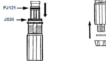
9. Replace injection stem into lower housing and attach 4 screws to base of lower housing.
