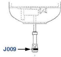
**!** To remove seal easily without tools, squeeze it on either side to raise the seal, then slide it over the groove. Using tools could damage the plunger.
