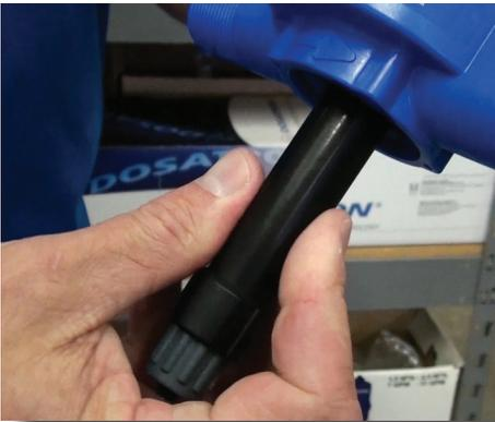
**Step 5:** Unscrew and remove the stem.
