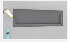
**Step 8.** Caulk all four sides of inlet after installation for improved inlet performance.
