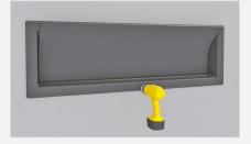
**Step 3.** Fasten 1 screw into center of bottom profile. Be sure it's straight across bottom.
