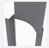
**Step 4.** Slide curved louver blade onto plastic hinge.
