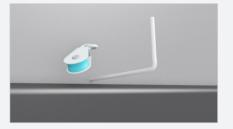
**Step 6.** Install winch block or pulley at the top of the inlet.
