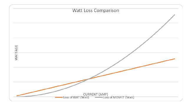
MOSFET losses are lower than IGBT losses until approximately 20 Amps.
