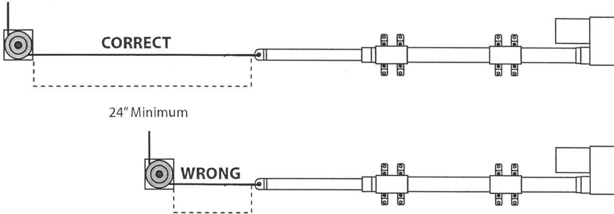
Pulley track must align on the same plane with actuator arm.
