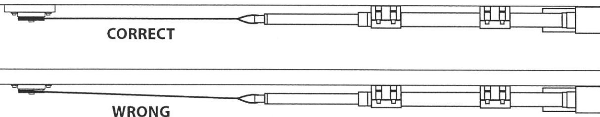
Pulley sets tracks must be no more than 1/2" apart and align with the actuator arm.
