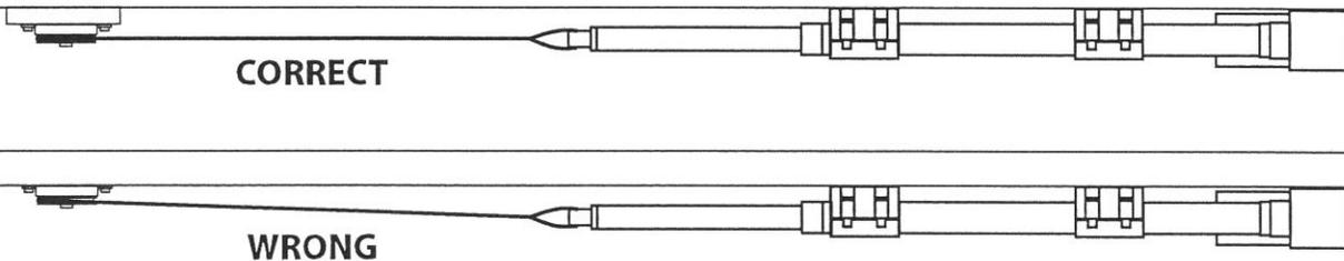
Pulley track must align with the actuator arm.
