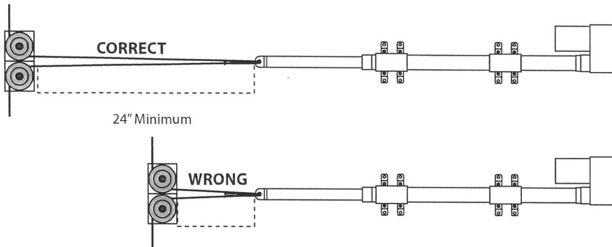
Pulley sets tracks must align on the same plane with actuator arm.
