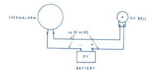
To assure complete reliability, it is essential that your alarm system be checked frequently. This may be accomplished by moving the set hands to the position of the temperature-indicating hand. If the alarm system does not trigger off, check all wiring to make sure that the connections are right and that the battery is charged. After testing, return the hands to the desired settings.
