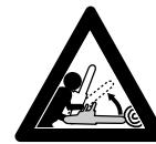
Kickback may occur when the moving saw chain near the upper quadrant of the bar nose contacts a solid object or is pinched.
