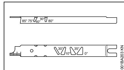
Use a STIHL filing gauge (special accessory, see table "Sharpening Tools"). This is a universal tool for checking the filing and side plate angles,
