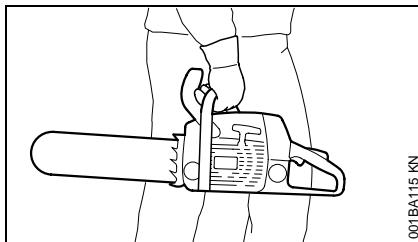
the fuel system is tight (no leaks) and that the controls and safety devices are working properly. Do not continue operating this machine if it is damaged. In case of doubt, have it checked by your STIHL servicing dealer.
