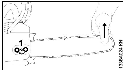
Retensioning during cutting work:
