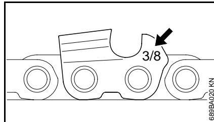
The chain pitch (e.g. 3/8") is marked on the depth gauge end of each cutter.
