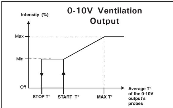
0-10V ventilation outputs start at their minimum intensity when the average temperature of their probes reaches the start temperature. They increase in intensity as the temperature increases; 0-10V outputs reach their maximum intensity when the temperature rises to the Maximum Temperature parameter setting.
