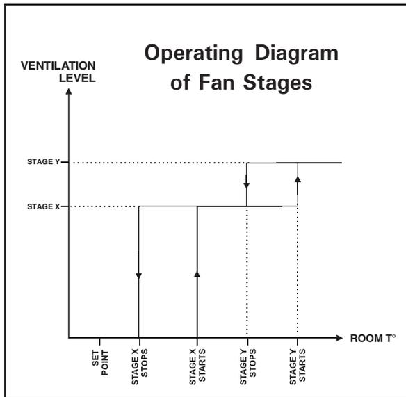
Start temperatures of fan stages are defined with respect to the set point and with respect to each other. This means that when one of these values is adjusted, all the consecutive values are adjusted by the same amount. For example, if the set point is increased by 1°F, the start temperature of all fan stages will be increased by the same amount.
