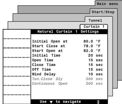
**Wind Delay** When the controller is in natural ventilation and temperature falls below the "Start Close At" temperature or rises above the "Start Open At" temperature, the curtain only starts moving after the wind delay has elapsed. This way, the curtain does not move when wind drafts cause sudden temperature changes. Set the wind delay to the desired value. Adjustable from 0 to 900 seconds (15 minutes).
