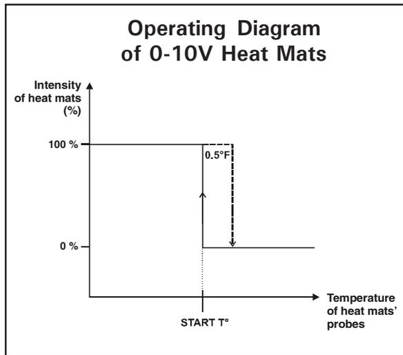
0-10V heat mats starts operating at its full intensity (100%) when the average temperature of chosen sensors reaches the start temperature of the output. It is disabled when the temperature rises 0.5°F (0.3°C) above the start temperature.
