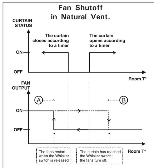
**Security:** If the temperature drops suddenly or if the whisker switch is defective, the controller automatically restarts the fans when the temperature falls 5°F (3°C) below the lowest curtain's closing temperature. When this situation occurs, a defective whisker switch alarm is posted to the alarm log.
