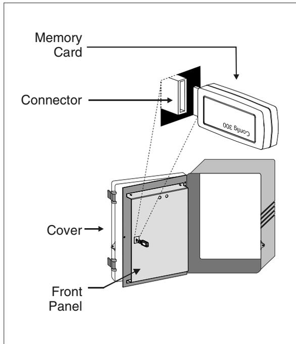
ware upgrade). The card can also be used to make a backup of your controller settings or to copy these settings on another controller of the same type.
