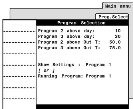
perature above which each program starts. Note that program 1 is automatically used when the animal age (or outside temperature) is lower than the value defined for programs 2 and 3.
