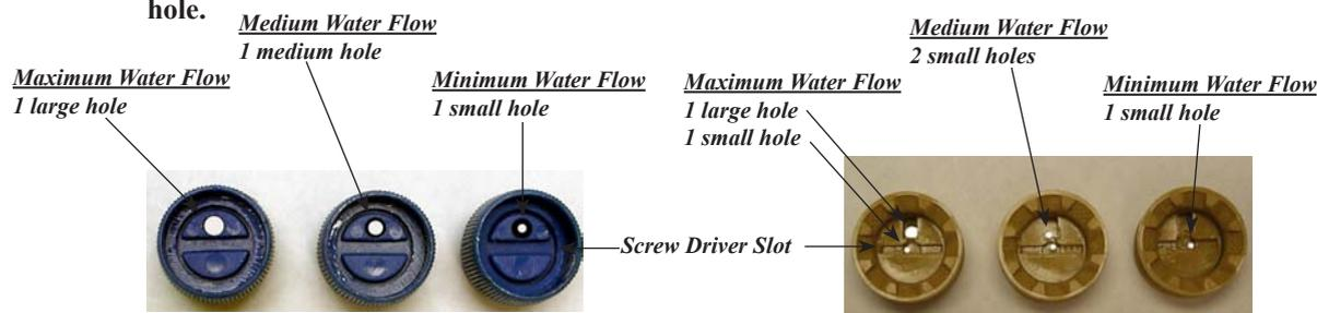
3. On the Gold Orifice, if you need to remove the orifice locate a quarter (25 cents). The quarter will fit very well into the grooves manufactured into the orifice rim. Turn counter clock wise with the quarter. After you remove the orifice the spring and trigger will fall out. The Blue Orifice you can remove by hand turning.
