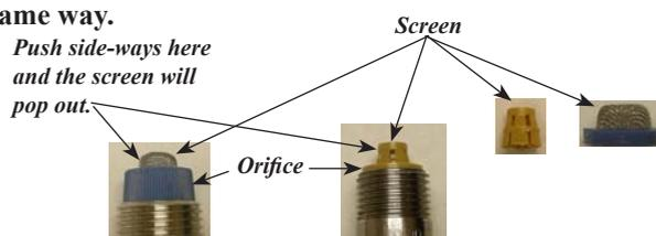
2. Looking into the orifice with the screen removed you will see a "Screw Driver Slot" in the middle of the orifice. You can adjust the water flow by turning the slot with your screwdriver. The slot is tight inside the orifice; it is manufactured this way to prevent the holes from being covered up by vibration moving the slotted disc. The nipples come from the factory set to the highest water flow setting, if you want to reduce the water flow you can turn the slot to a smaller hole.
