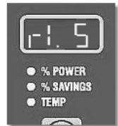
After 20 seconds of keypad inactivity, the control will return to the normal display.
