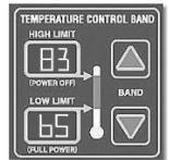
After 20 seconds of keypad inactivity, the control will return to the normal display. (Note: only the LOW LIMIT is changed during this process. To change the HIGH LIMIT, adjust the temperature setting as described in the previous section).
