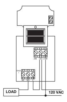
Figure 4: Typical 120 VAC Wiring Diagram.
