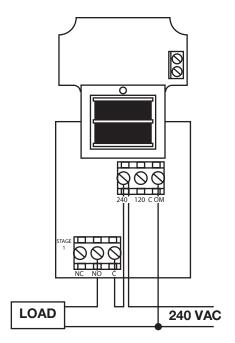
Figure 5: Typical 240 VAC Wiring Diagram.
