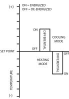
Figure 1: Setpoint and Differential Settings. Diagram indicates relay on and off points in either the heating or cooling modes.
