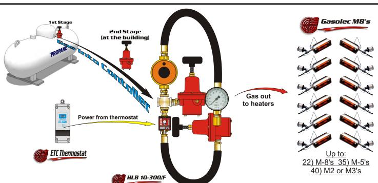
The HLB10-300F GAS CONTROLLER is designed to provide the most economical and efficient use of gas, while maintaining optimum bird comfort. It allows your Gasolec brooders to operate fully within their designed ranges, from a pilot or maintenance heat of 20 mbar (0.3 psi) to their maximum of 300 mbar (4.5 psi).
